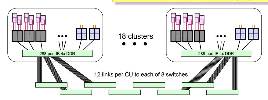
Eight 2<sup>nd</sup>-stage 288-port IB 4X DDR switches
