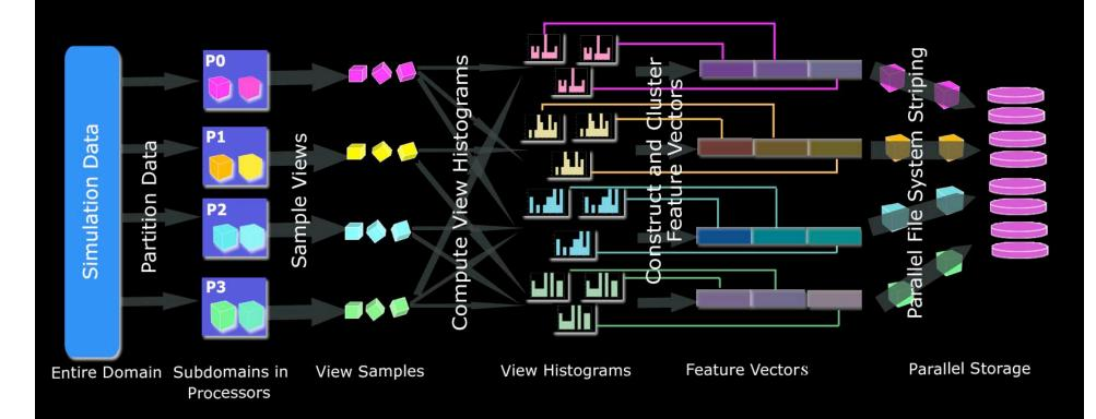
Algorithm overview consists of: partitioning data, sampling views on a view sphere, computing view histograms for each view direction, concatenating view histograms into feature vectors, grouping similar feature vectors into clusters, and striping data blocks onto parallel storage according to the clusters.
