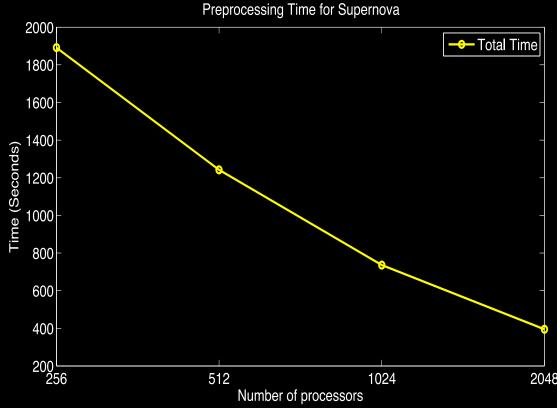
Total preprocessing time for supernova dataset, from 256 to 2048 cores, on Argonne's BG/P system. The dataset is 276 GB, and 1024 views were sampled in under seven minutes.
