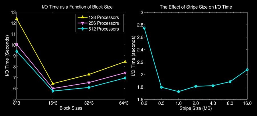
Block size of 16<sup>3</sup> has best I/O performance for Viswoman dataset, irrespective of process count. Block size is chosen to be a multiple of the read buffer size, 16 KB in our default MPI-IO implementation.
