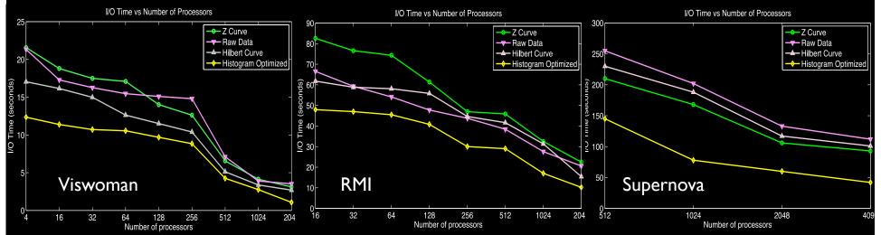
Top: I/O time for three datasets. Bottom: compositing, rendering, I/O time for supernova. In all test cases, the histogram-optimized method performs better than canonical organization and space-filling curves.
