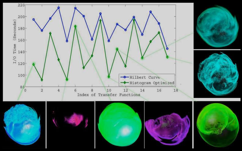
I/O time for histogram-optimized and Hilbert curve for supernova dataset rendered with a variety of transfer functions. Transfer functions were generated synthetically using a nonlinear computation that stochastically produces one or more modes.
