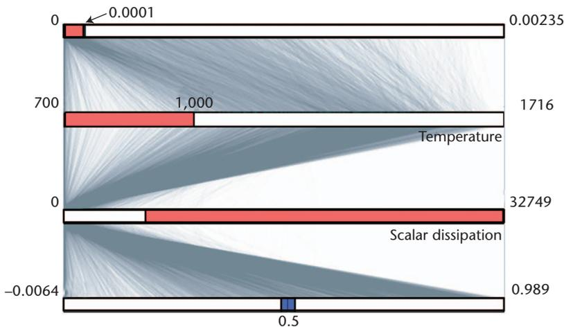
Figure 8. The multivariate data visualization interface. We use this interface to extract a feature involving four variables: OH, temperature,  $\chi$ , and a mixture fraction. Figure 9 shows the resulting visualizations.
