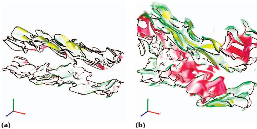
Figure 4. Nonphotorealistic rendering of three variables. At (a) time step 11, and (b) time step 41, we see different views of OH (red),  $\chi$  (yellow and green), and a mixture fraction isosurface.
