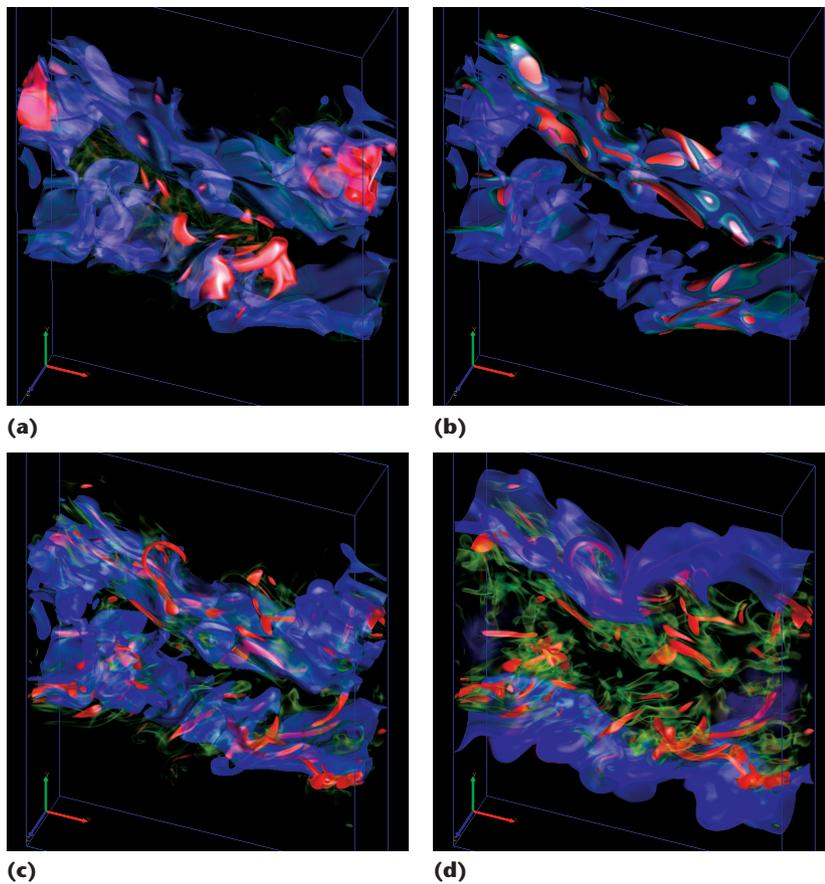
**Figure 1. Simultaneous visualization.** (a) The mass fraction of the hydroxyl radical, OH (red), and stoichiometric mixture fraction isosurface (blue); (b)  $\chi$  (red/yellow) and a mixture fraction (blue); (c) vorticity (red/yellow) and a mixture fraction (blue); and (d) vorticity (red/yellow) and heat release (blue). All the images are for time step 41. Except for the mixture fraction isosurface using  $\text{isovalue} = 0.5$ , all others emphasize high values.
