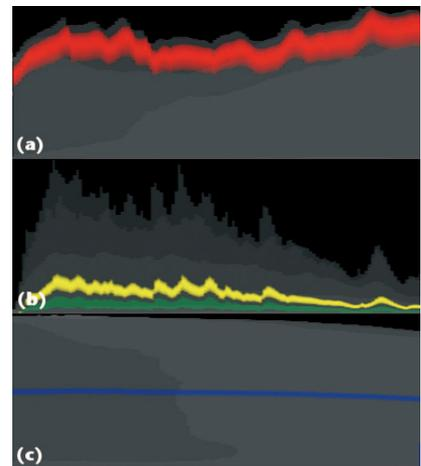
**Figure 6. Time-histogram interface showing data distributions and trends in the temporal domain. The x-axis is time and the y-axis is data value. The shade of each pixel indicates the number of occurrences for the corresponding value at the corresponding time step: (a) OH, (b)  $\chi$ , and (c) a mixture fraction. The colored regions correspond to the visible flow features in the visualization.**
