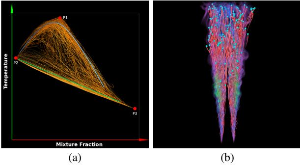
Figure 1: (a) shows the time series curves representing correlation between temperature and *mixture fraction*, which are two key parameters in the combustion simulation of a turbulent lifted autoignitive ethylene/air jet flame. There is a great deal of clutter and it is hard to perceive detailed correlation patterns. (b) shows the corresponding particle trajectories in the physical space, with volume rendering of the hydroperoxy field.
