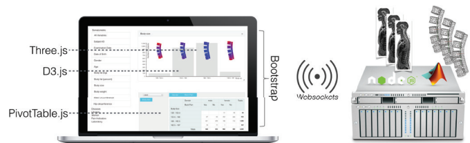
Fig. 5. The front-end solution (left) uses HTML5/CSS3 , WebGL and SVG to display the data. The NodeJS based back-end (right) stores all image and non-image data and transfers it to connected clients. All computation-heavy operations, such as calculation of mean shapes or distances, are performed on the server side. Client-server communication is accomplished via the Websocket protocol.
