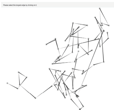
Fig. 7. Screenshot of an example of Task 2 (longest link). Tapered links (T) with node splatting (SP) and depth sorting (LF) is used. The legend at the top contains the question.
