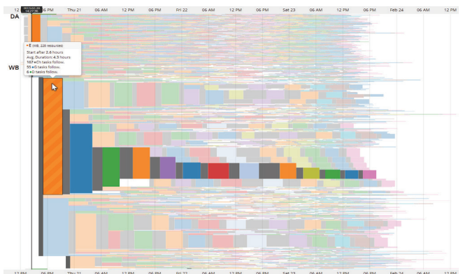
Fig. 7. LiveGantt can visualize a huge schedule which comprises 18,577 tasks and 500 machines. Resources which have very similar task sequences are represented by rainbow-striped horizontal bars.
