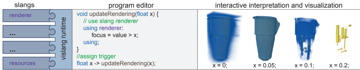
Fig. 1. System Overview: Slangs are DSLs that encapsulate a certain functionality and register it with the ViSlang runtime. The ViSlang runtime implements an embedded interpreter that executes programs in an interactive environment. The user interacts with an integrated program editor to issue ViSlang commands.
