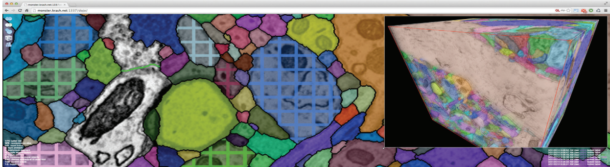
Fig. 1: Proofreading with Dojo. We present a web-based application for interactive proofreading of automatic segmentations of connectome data acquired via electron microscopy. Split, merge and adjust functionality enables multiple users to correct the labeling of neurons in a collaborative fashion. Color-coded structures can be explored in 2D and 3D.
