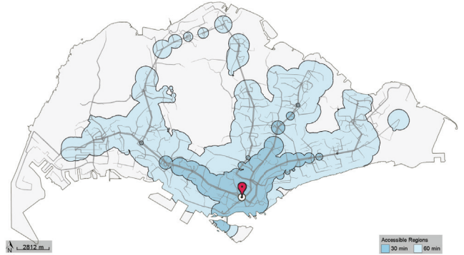
Fig. 5. The isochrone map view presents spatial-reachability regions from 8am at origin A (red icon), which is station WW16/YY3 in the city center, by contour lines and areas over the geographical map. Dark blue and light blue indicate [0, 30] and (30, 60] minutes, respectively.
