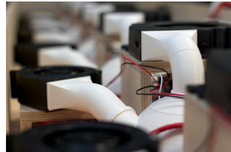
Figure 6: Arduino controlled fans and 3D printed housing
