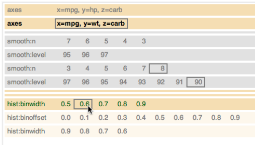
Figure 2: History Rewind. In the session shown in Figure 1, the user adjusted parameters for a smoothed line, then switched off the line and switched on a histogram. Here the ephemeral history rewind is being used to revisit the first time the histogram bin width was set to 0.6. History items in the future are shown in a lighter colour: for example, here the bin-offset slider has yet to be moved from its default initial value of 0.
