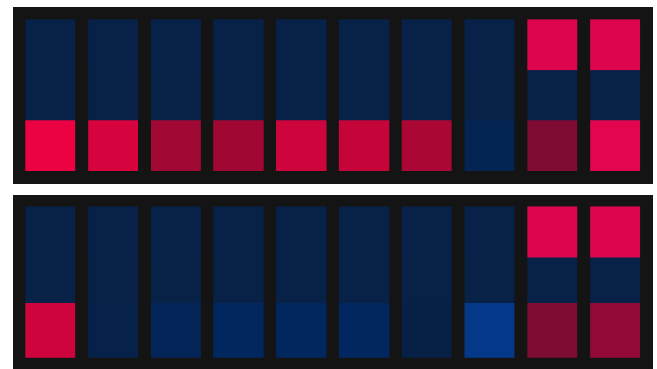
Fig. 7: Effects of “binning” different values of a parameter together. In this case, we instructed the color mapping to treat all jpeg images (as part of the URL ) as if it was one and the same. While each image on its own is rarely accessed (indicated by red pixels in the top band), jpegs in general are a usual request (blue pixels in the bottom band).
