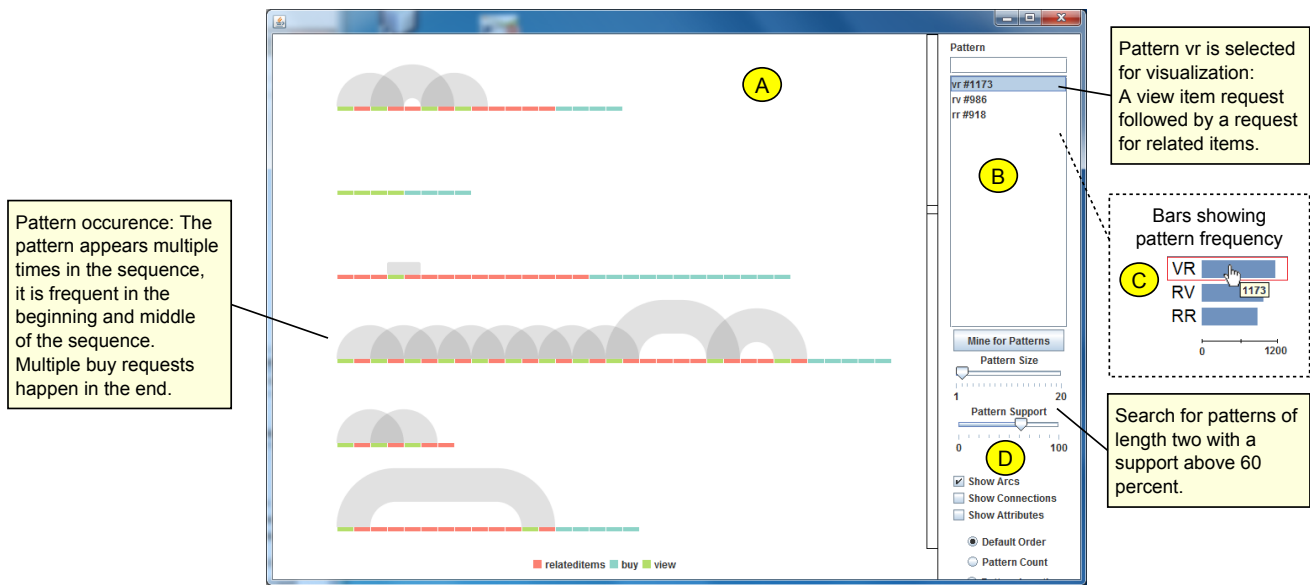
Figure 2: Design prototype. The screenshot shows a part of the example event log. (a) The visualization of event sequences together with a recurring event pattern. (b) List of mined and manually entered event patterns. (c) Pattern frequency shown by horizontal bars. (d) Patterns of a defined length and support value can be mined automatically.
